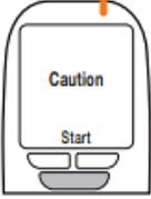
You must acknowledge that alcohol has been detected by pressing the bottom navigation button before starting the vehicle engine.
