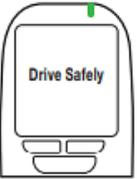
**b.** If the status light is solid amber and the handset displays **Drive Safely**, alcohol was detected below the FAIL set point. You may continue to drive the vehicle.
