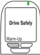
**2. Warm-up** is displayed and the vehicle engine can remain idling without requiring another breath test for the prescribed period of time (default is 30 minutes).
