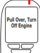
You must safely park the vehicle and turn the ignition off. **Hold Right Button to Cancel Restart** will display on the handset. Press the right navigation button to cancel the restart option.
