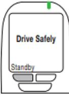
**Standby** is displayed and the vehicle engine can remain idling without requiring another breath test for a prescribed period of time (default is 30 minutes).
