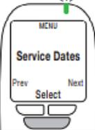
**3.** Press the left or right navigation button to scroll through all the dates. Press the bottom navigation button to exit this menu.
