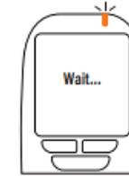
1. Power on the device by pressing any navigation button. The status light will flash amber. The handset will display **Wait...** until the device warms up.
