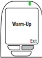
After the prescribed period of time, the **Warm-Up** mode automatically ends, or manually exit **Warm-Up** mode by pressing and holding the right button or pressing the accelerator pedal.
