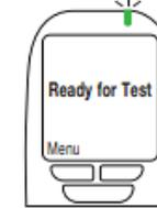
2. The status light will flash green and the handset will display **Ready for Test**. The warm-up time may be longer in cold temperatures.
