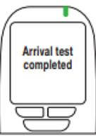
**b.** If alcohol is detected below the FAIL set point, the status light will be solid amber to indicate caution and the handset will display **Arrival test completed.**
